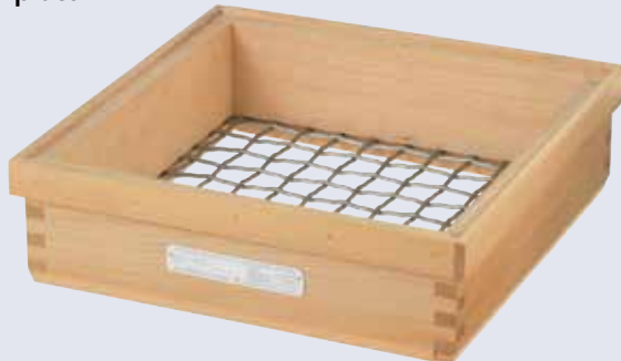
Test Sieve with beechwood frame
